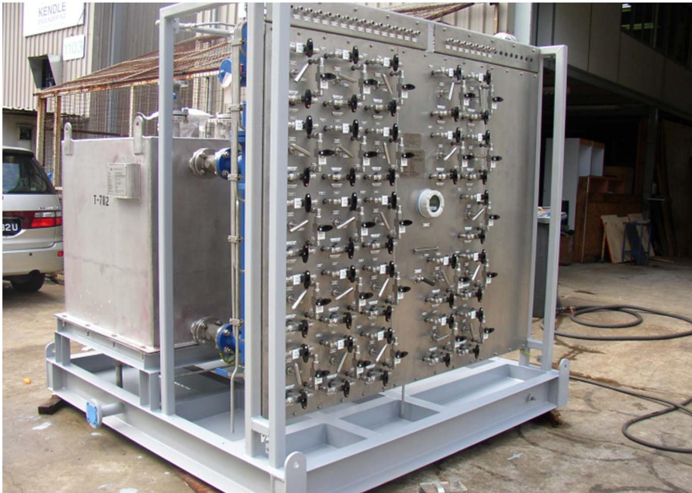
**Corrosion Inhibitor Skid Package for GSPC – NIKO Resources Ltd**
