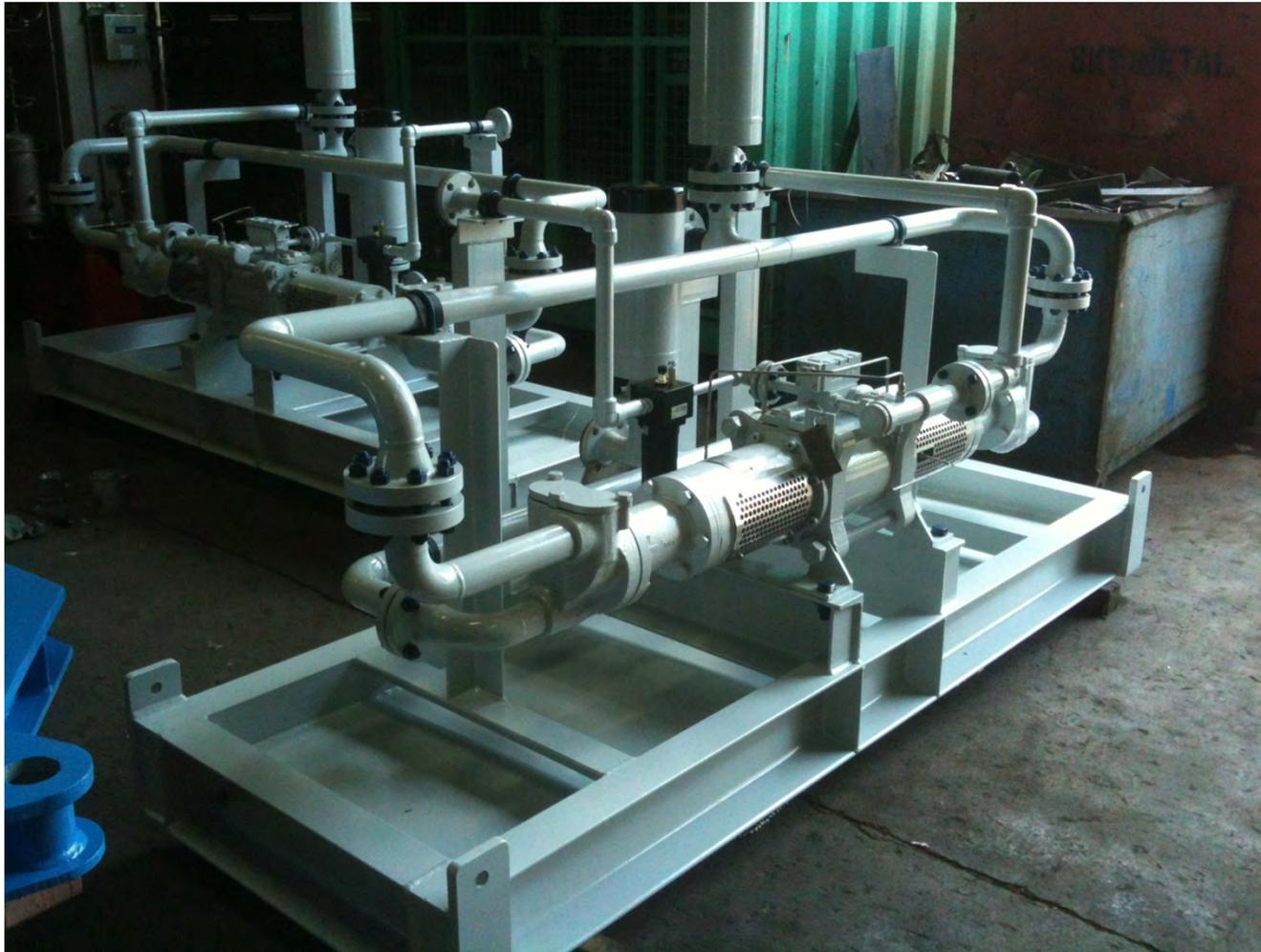
**Closed Drain Sump Pump Skid for CPOC**
